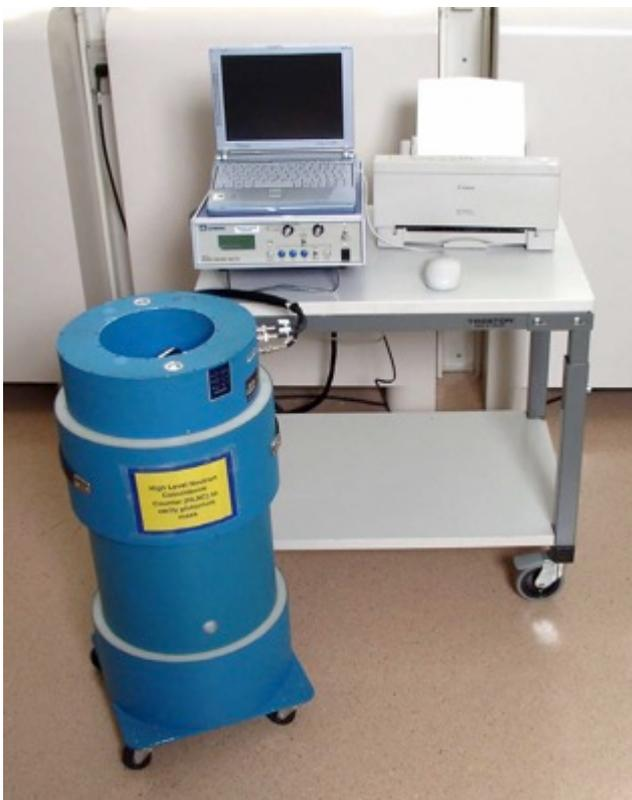
**High-level neutron coincidence counter, HLNC, used to measure plutonium mass in combination with a determination of Pu isotopes.**
