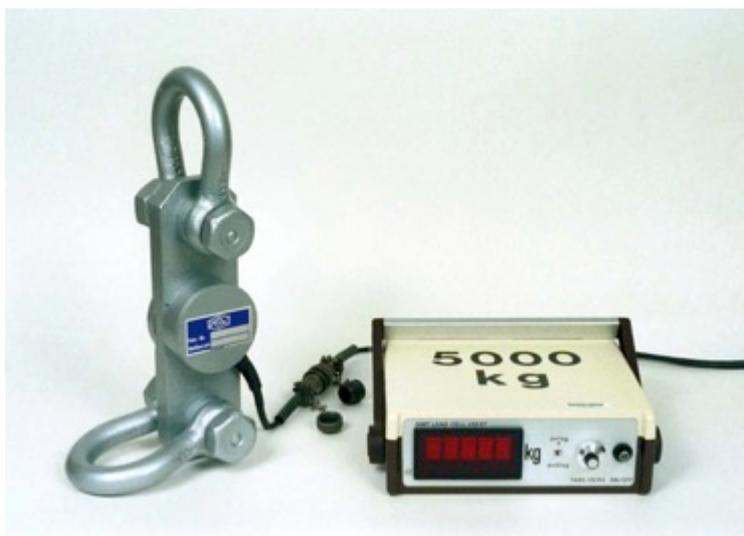
**Load cell based weighing system with a capacity of 5000 Kg.**
