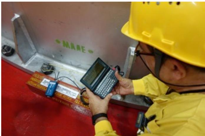
**A VACOSS seal being attached by an IAEA inspector
