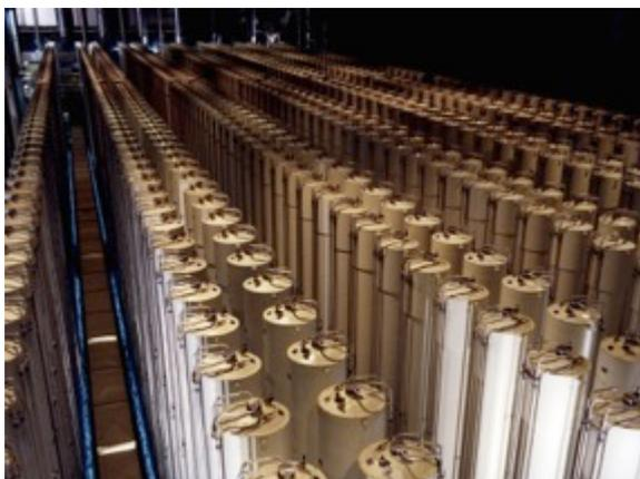
**Cascade of gas centrifuges used to produce enriched uranium.**
