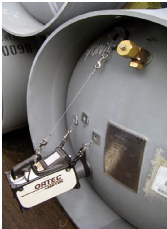
**An electrically cooled germanium system used to verify the enrichment of UF<sub>6</sub>.**
