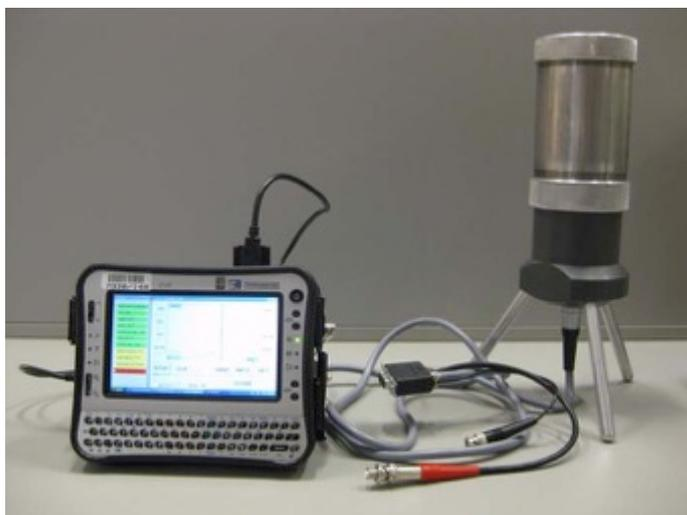
**Miniature multichannel analyzer with NaI detector and portable computer.**
