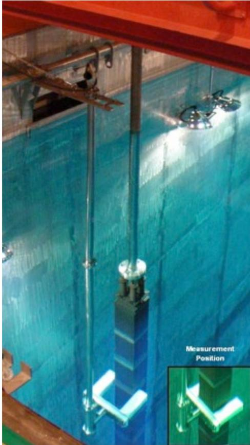
**A Fork detector measuring a spent fuel assembly at a reactor pond.**
