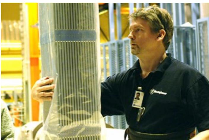
**A PWR fuel assembly ready to be shipped to a reactor.**
